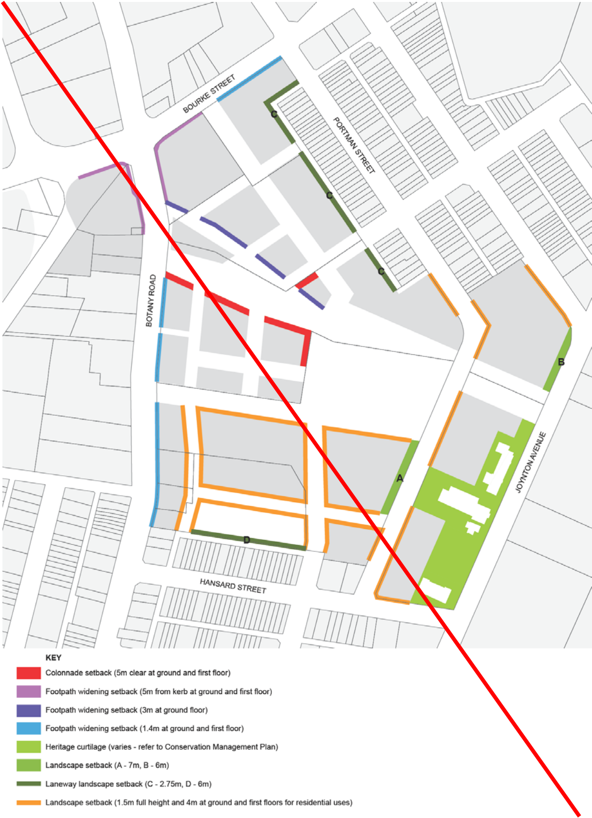
Figure 6.14: Street frontage alignments and primary setbacks
